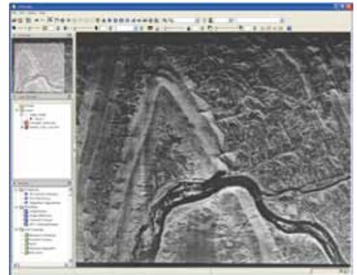
Fig. 3: Radar and data fusion tools in ENVI are especially useful when an area of interest is inaccessible or obscured by clouds in optical imagery.
