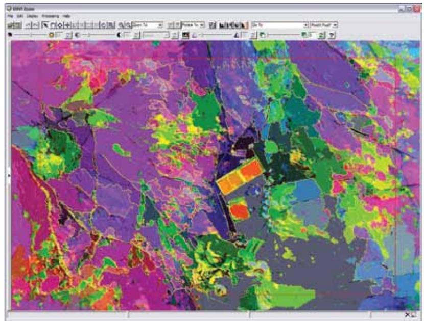
Fig. 1: ENVI feature extraction can be used to separate unique geologic regions to identify viable mining and drilling sites.
