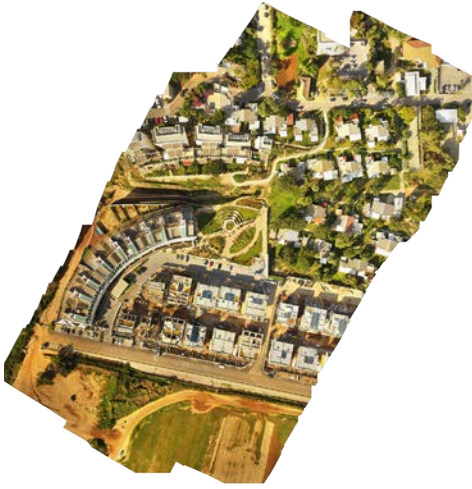
Orthomosaic of a residential housing subdivision shot from DJI Phantom. Total time to process was 49 minutes.
