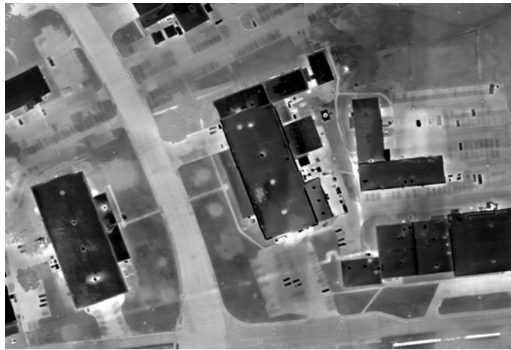
Thermal orthomosaic of a corporate campus showing pipes down to 2 meters underground.
