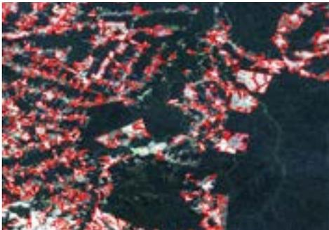
*When the workflow is complete, the results are output as a vector file, which can be used in both ENVI and ArcGIS for further analysis and to create an output map.*
