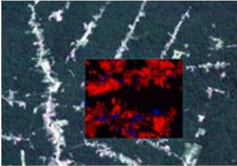
*This image previews ENVI change detection results. Using two Landsat images taken at different times, ENVI automatically identified deforested areas (in red). The blue areas indicate new growth/planting.*
